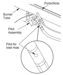
Figure 44 - Pilot Inlet Air Hole
